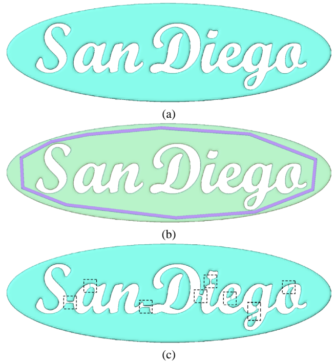
Figure 9: An example of topology design: the source model (a) (a plate with words “San Diego” carved out) is different from the target (purple in (b)) in both the number of handles and islands. After editing, both the plate and the words become a single connected component (c). Editing involves both subtraction (for breaking handles) and addition (for bridging islands), highlighted in (c), to guarantee a topologically consistent result with minimal change.
