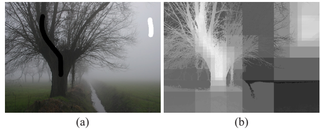
Figure 2: Adaptive clustering in affinity space. (a) An image with two user strokes. (b) Pixel clusters colored by their distances to the closest user-edited pixel in the affinity space. Note that clusters further away from the strokes, which are dimmer, have larger sizes.
