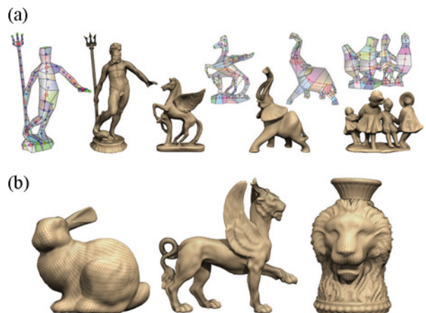
Figure 5. (a) Constructed poly-pipes and semi-regular quadrilateral meshes of four models with non-zero genus. (b) Models used in comparison with Ray et al. [2].
