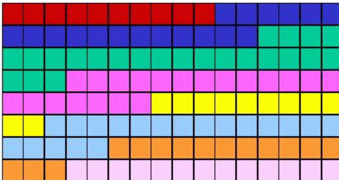
Figure 2: A possible slice structure for a frame
