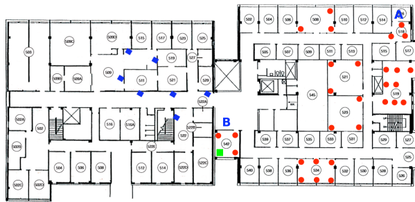
Figure 1. Circles denote relay nodes that are part of testbed. Diamonds indicate relay nodes plugged into wall outlets. A square denotes the base station. Positions A and B are used in the mobility study.
