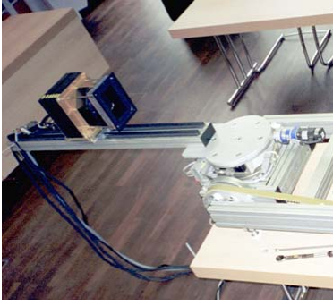
Figure 4: Line-based panoramic camera at the Institute of Space Sensor Technology and Planetary Exploration, German Aerospace Center (DLR), Berlin.
