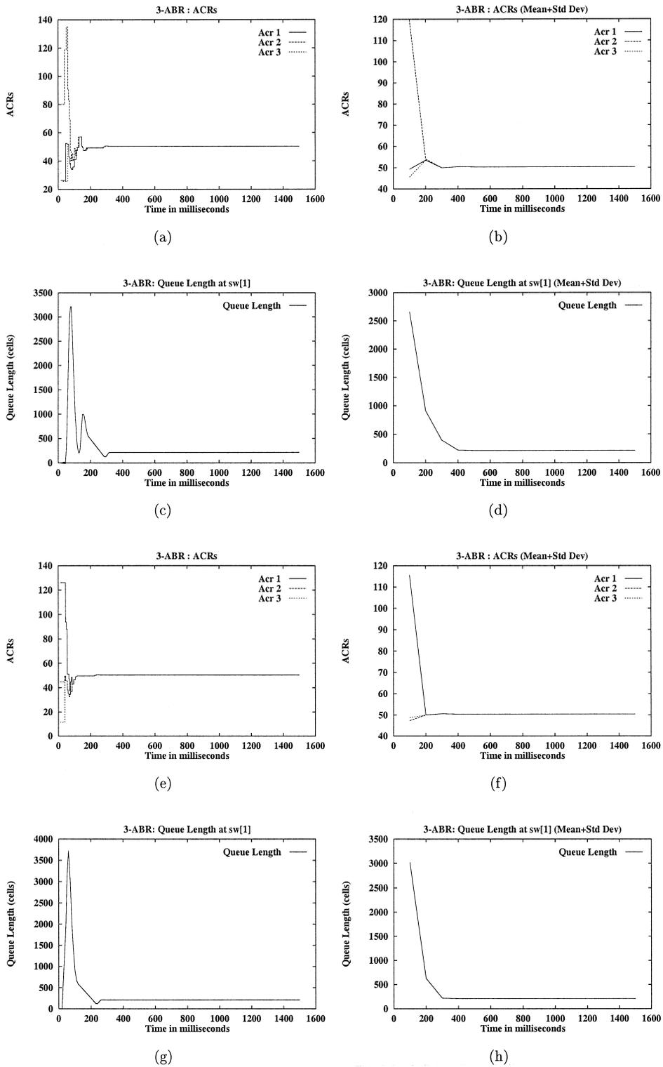
Fig. 5. Simple configuration: rate and queue graphs: hyperbolic and inverse hyperbolic queue control function.
