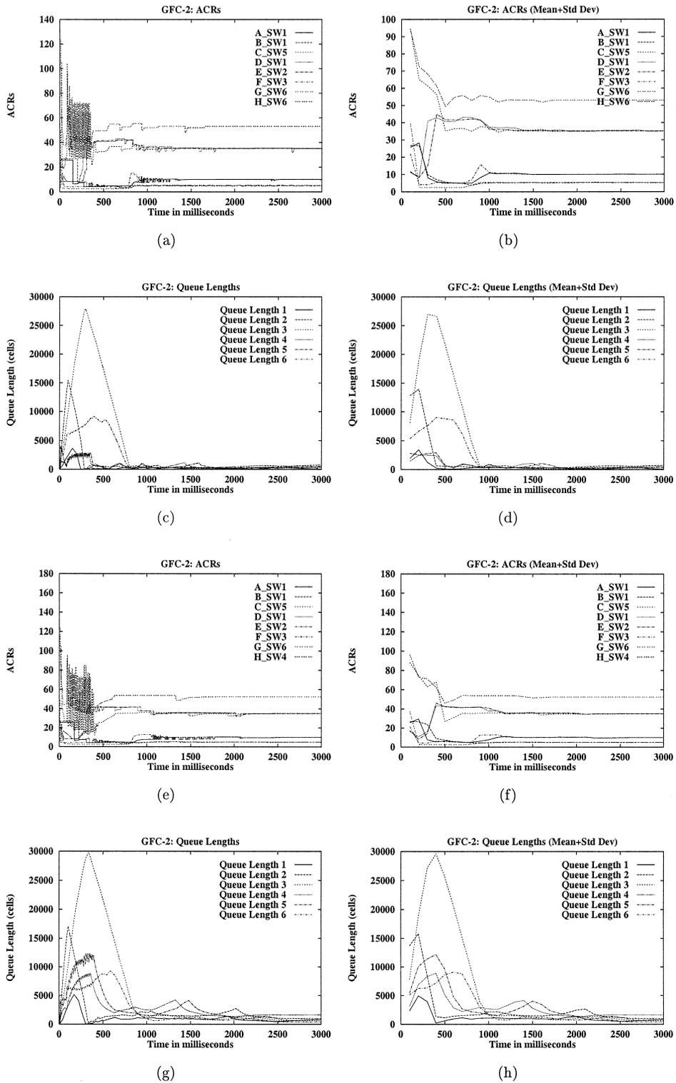
Fig. 7. GFC-2 configuration: rate and queue graphs: hyperbolic and inverse hyperbolic queue control function.
