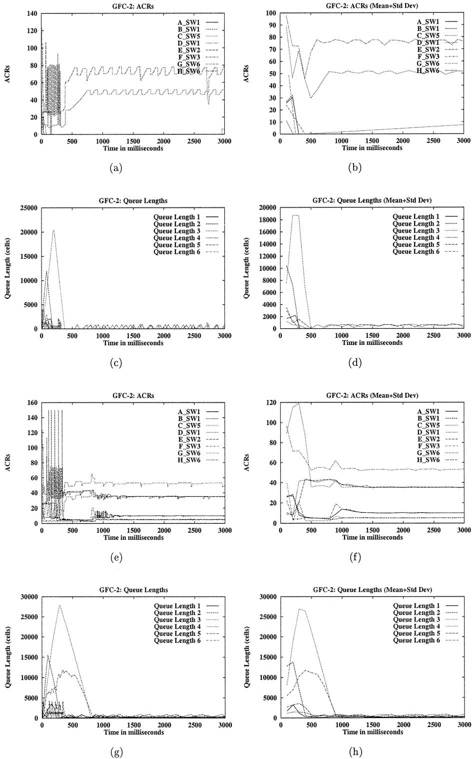
Fig. 6. GFC-2 configuration: rate and queue graphs: step and linear queue control function.
