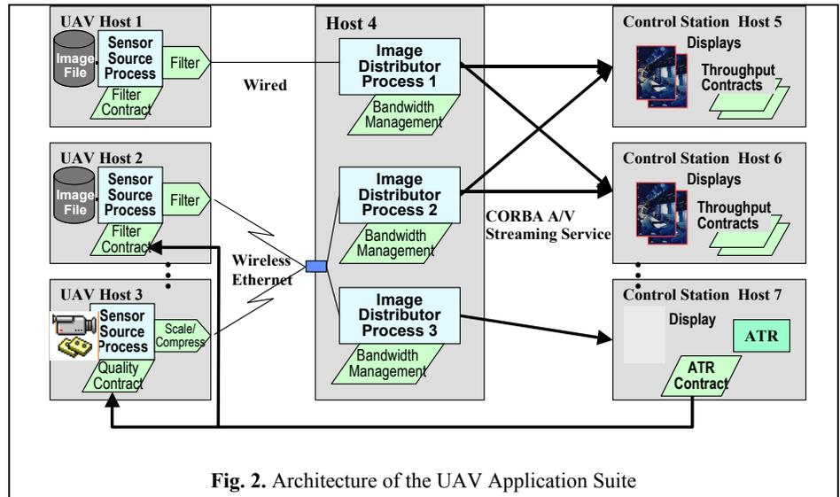
Fig. 2. Architecture of the UAV Application Suite
