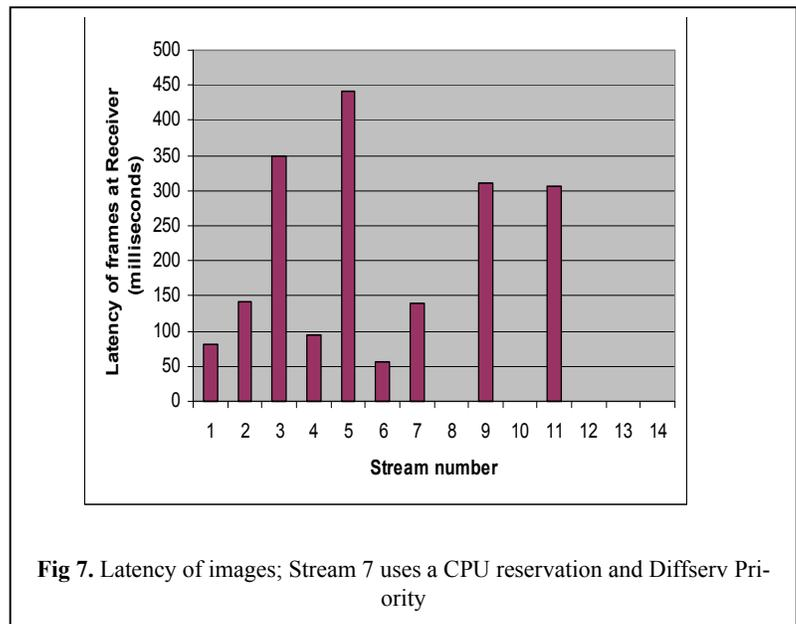
Fig 7. Latency of images; Stream 7 uses a CPU reservation and Diffserv Priority
