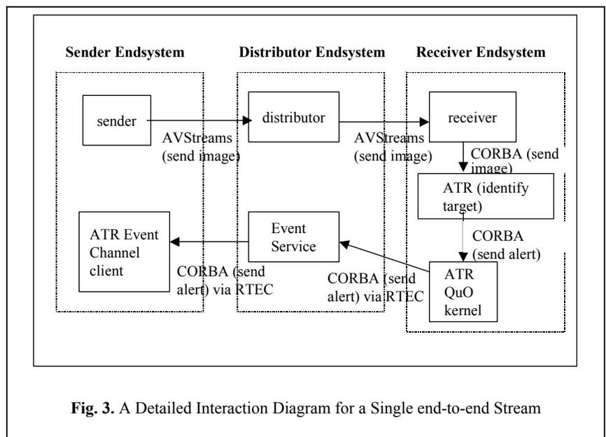
Fig. 3. A Detailed Interaction Diagram for a Single end-to-end Stream
